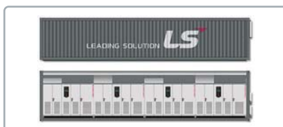
Internal configuration (4MW per 40ft container)
